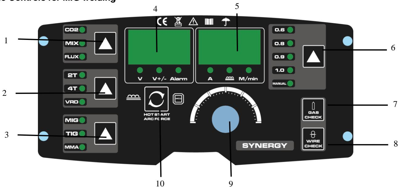
5.1.5.1 Gas selection: CO2--ordinary CO2 gas; MIX--20% CO2 80% argon; FLUX-- flux cored
