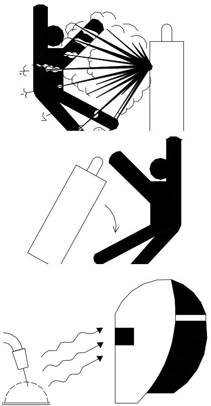
**Note:** Since the arc of MIG welding is much strong than that of MMA welding, please wear welding helmet and protective clothing.
