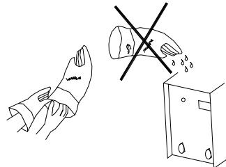
7. To avoid water and rain, if there is, dry it in time, and check the insulation with mega-meter (including that between the connection and that between the case and the connection). Only when there is no abnormal phenomenon should the welding continue.
