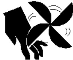
5. Clear the dust at regular intervals with clean and dry compressed air; if the working condition is with heavy smoke and air pollution, the welding machine should be cleaned daily.
