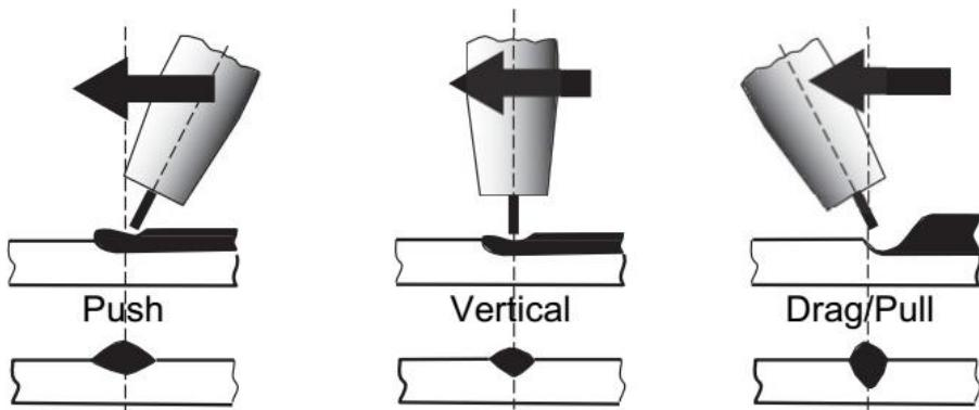
The welding gun should be held at an angle to the weld joint. (See Secondary Adjustment Variables below) Hold the gun so that the welding seam is viewed at all times. Always wear the welding helmet with proper filter lenses and use the proper safety equipment.
