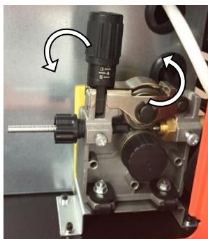
5.1.2.2 check the wire drive roller(21) groove matches the selected MIG wire type and size. The drive roller will have two different sized grooves, the size of the groove in use is stamped on the side of the drive roller. For flux cored 'soft' wire ,such as that used in gasless MIG welding, the drive roller groove has a serrated profile. For solid 'hard' MIG wire, the roller groove has a 'v' shaped profile
